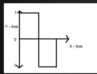
The signal has been quantified into three different levels
