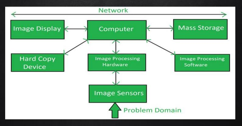
**Image Sensors:** Two elements are required to acquire digital images, the first is a physical device that is sensitive to the energy radiated by the object we wish to image. The second is a digitizer, which is a device for converting the output of the physical sensing device into digital form.
