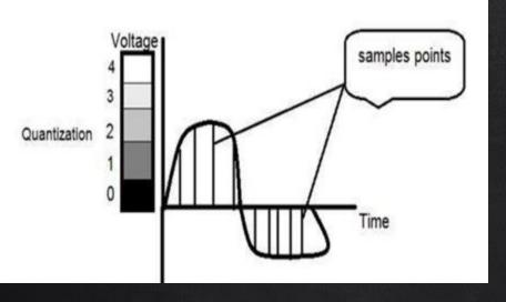
Signal has been quantized into 5 different levels or partitions. Ranging from 0 black to 4 white.
