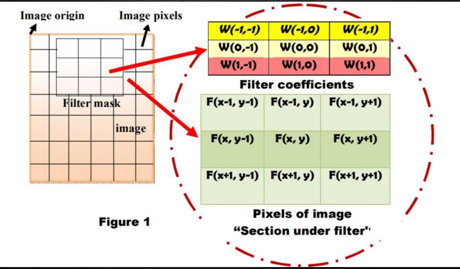
Observe that the center coefficient of the filter, w(O, O) aligns with the pixel at location(x, y).
