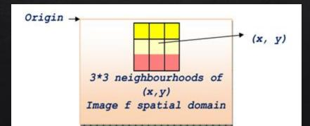
Filtering creates new pixels with coordinates equal to the coordinates of the center of the neighborhood, and whose value is the result of the filtering operation.
